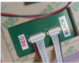
**Step 4: Peel the adhesive and precisely apply the touchpad.**
